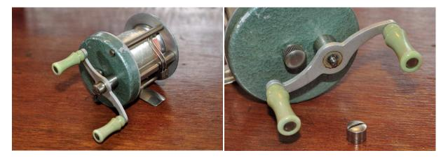
This is a very simple reel to service with very few moving parts. Start by removing the handle nut and handle.
