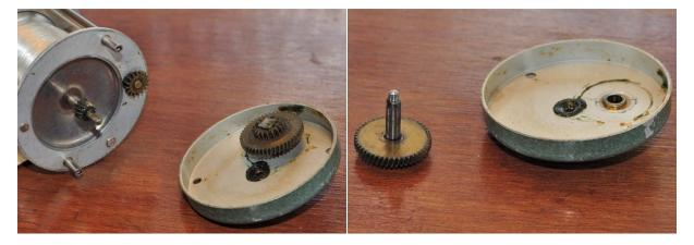
Remove the plate from the frame and remove the main gear from the side plate, it simply lifts out.
