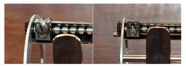
The level wind assembly comes apart in typical ABU fashion; undo the screw at the base of the line carriage and remove the pawl.
