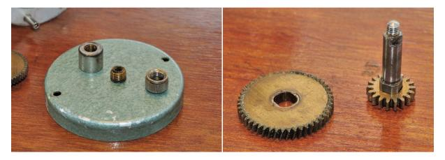
At this point you can remove the spool cap and add a drop of oil. The main gear separates from the shaft, the gear at the base of the shaft turns the level wind worm gear.
