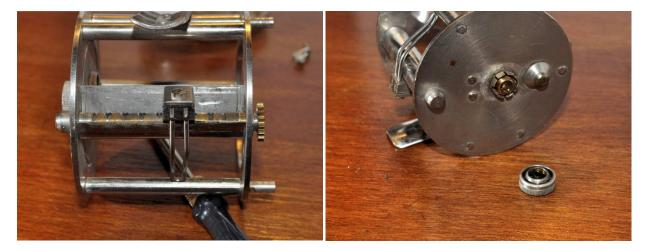
The level wind assembly is removed in typical ABU fashion; remove the screw and cover on the line carriage and then remove the pawl. The worm gear can then be removed from the side of the frame. Unscrew the spool cap on the left side plate and add a drop of oil.
