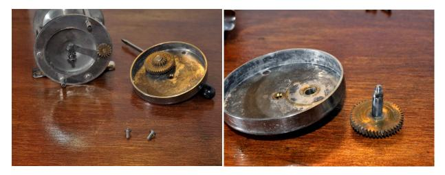
Undo the two pillar screws and remove the right hand side plate. The main gear simply lifts out of the side plate.
