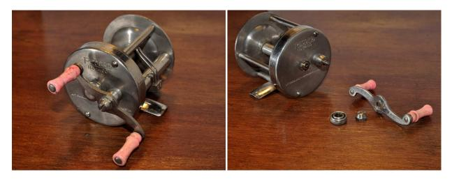
Start by removing the handle nut and handle. Remove the spool cap and add a drop of oil to the felt.
