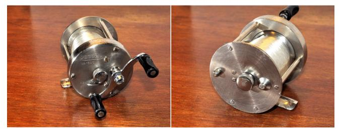
Before reassembly give everything a thorough clean. Add grease to the gears and all screw threads (to stop them seizing), and a light oil to all other friction surfaces.
