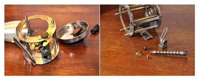
The level wind assembly removes in typical ABU fashion; remove the retaining clip on the right side of the frame, undo the pawl cover and remove the pawl, and then the whole assembly can be removed from the right hand side of the frame.
