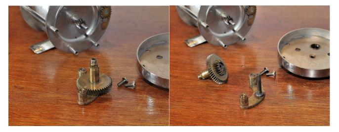
The bridge assembly can then be removed from the side plate. Tthe main gear simply lifts off the bridge assembly.
