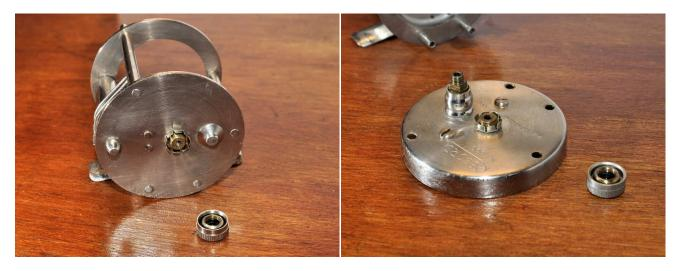
Remove both screw caps and add a drop of oil. Remove the two bridge screws on the right side plate.
