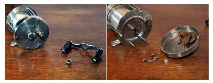
Remove the handle nut and handle. Undo the four pillar screws and remove the side plate from the frame.
