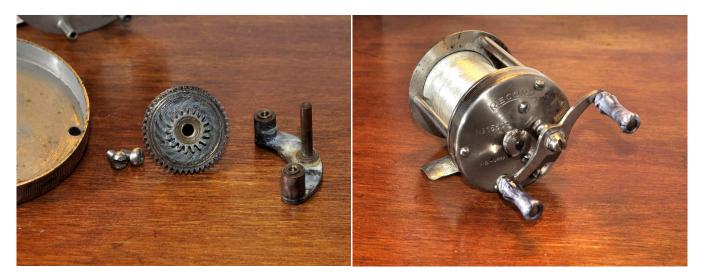
The main gear lifts off the bridge assembly. Give everything a thorough clean before reassembly.
