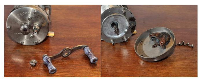
Start by removing the handle nut and handle. Remove the four pillar screws and lift off the side plate.
