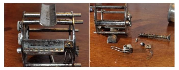
The level wind removes in typical ABU fashion; undo the screw and remove the pawl cover and pawl. Remove the worm gear retaining clip from the right side of the frame and then the whole level wind assembly can be removed.
