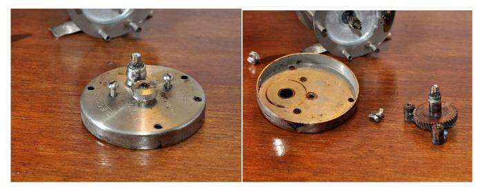
Two bridge screws hold the bridge assembly and gears in place on the right side plate. Remove these screws and the bridge assembly simply lifts out.
