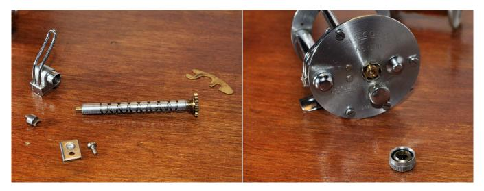
The whole assembly can then be removed from the right side of the frame. Add a drop of oil to the spool caps.
