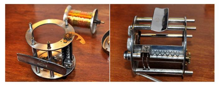
To remove the level wind assembly first remove the retaining clip, then unscrew the pawl cover and remove the pawl.
