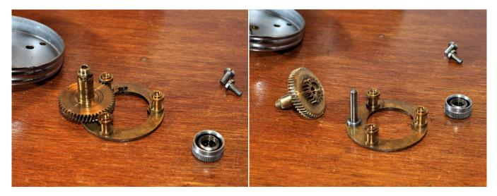
The gears simply lift off the bridge assembly.
