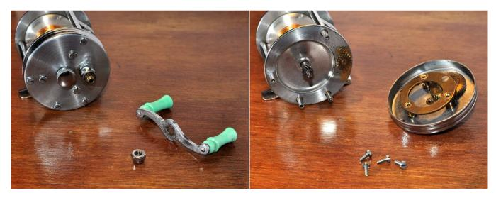
Remove the handle nut and handle. Remove the four pillar screws and lift off the right side plate from the frame.
