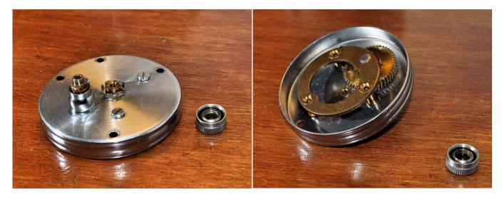
Undo the three bridge screws and remove the entire bridge assembly from the right side plate.
