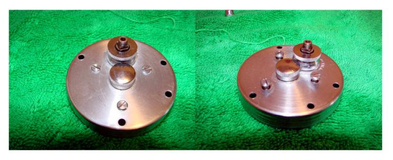
Lift off the side plate and undo the remaining three screws on the side plate. These attach the bridge to the side plate. The spool can be removed from the frame at this time.
