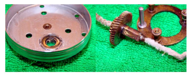
Lightly coat the washers with drag grease and replace in the right side plate making sure that the retaining clip is seated fully. In this photo there is actually a lot of grease! A pipe cleaner dipped in lighter fuel is great for cleaning the inside of the main gear.
