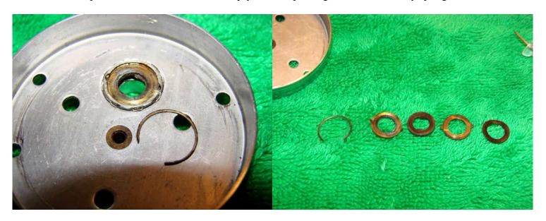
The washers can then be removed. The order here is left to right =bottom to top (I have called the washers with 'ears' keyed washers). Split ring, keyed washer/fibre washer/keyed washer/spring washer. The fibre washer that sits on the main gear is not shown.
