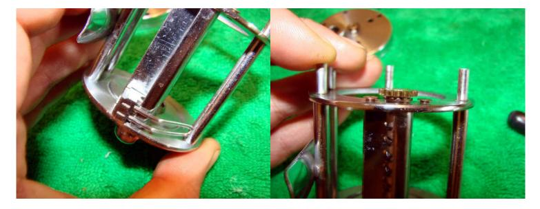
Place the level wind so that it sits in the left side plate-this makes it easier when replacing the worm gear. Note in the above picture that the bushing is not yet flush with the frame.
