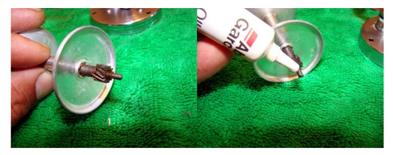
As will the right side. When clean add a drop of oil to the shaft where it contacts in the side plate (both sides), and some grease to the pinion gear.
