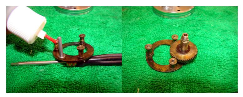
Smear some liquid grease on the post for the main gear ensuring complete coverage and then replace the main gear. Add a light coating of drag grease to the fibre washer before replacing on top of the main gear. Add a light smear of grease to the three posts on the bridge where they contact the side plate.
