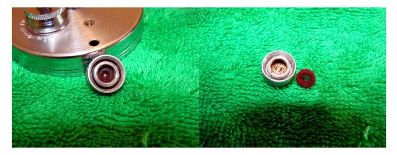
Remove the spool cap from the right side plate. There is a little bit of corrosion in the red felt washer that has come from the spool shaft. Very carefully pry out the felt washer. A wooden toothpick is good as it will not scratch. Be aware that the felt is old and may be delicate.
