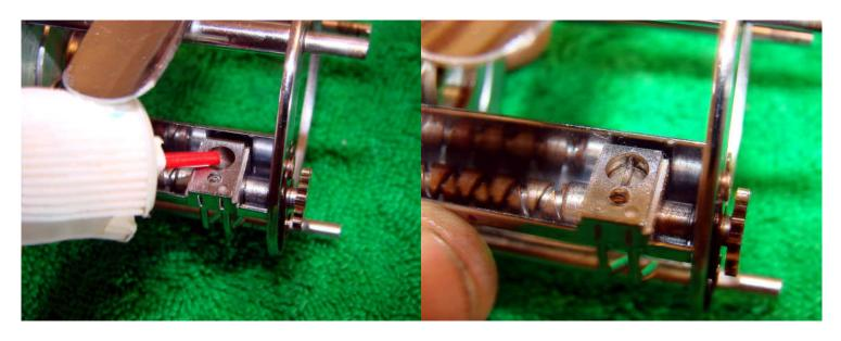
Add a drop of oil or liquid grease to the inside of the level wind before replacing the pawl. Make sure that it seats properly in the grooves on the worm gear-do not force!
