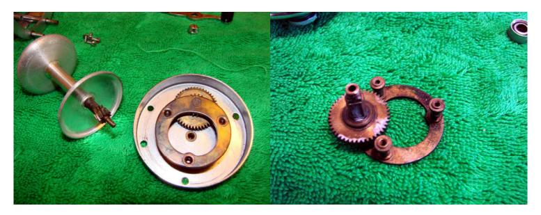
Turn the side plate over and remove the entire bridge assembly with the main gear attached. Note the fibre washer that sits on the main gear.
