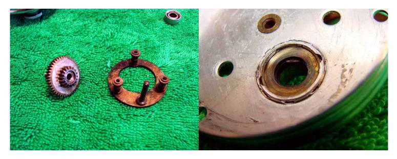
The main gear lifts off the bridge. The washers in the side plate are held in by a split ring (locking washer). Note the two slots. Use a pin or similar tool in the slots to pry out the split ring-take care as it may spring off.
