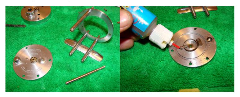
Note that one of the frame bars is not attached to the frame. Add a drop of liquid grease to the clicker assembly-if you work the clicker button backwards and forwards (other side of side plate) it will ensure proper coverage. Add a drop of grease to both sides of the click hammer where it contacts the click spring.
