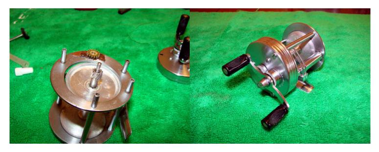
Place the spool back in the frame and then reattach the right side plate. Replace the four (greased) pillar screws. Adjust the spool caps so there is barely discernible side to side play i.e. they are lightly touching the ends of the spool shaft.
