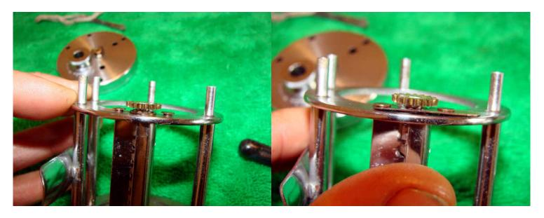
The bushing will need to be pushed flush with the frame before the locking washer can be replaced.
