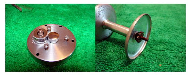
Place the whole bridge assembly back in the side plate and then replace the three bridge screws-remembering to grease the threads! The left side of the spool shaft will need to be cleaned up.
