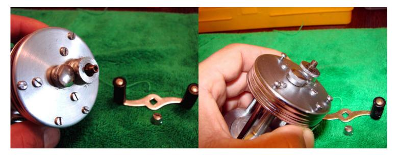
Starting on the right side plate (called head cap on the schematic), remove the handle nut and the handle. Undo the four pillar screws holding the side plate to the frame-the importance of having properly fitting screwdrivers cannot be overstated. Nothing makes a reel look old quickly as mangled screw slots. It is nice to note that the threads on these screws are greased.
