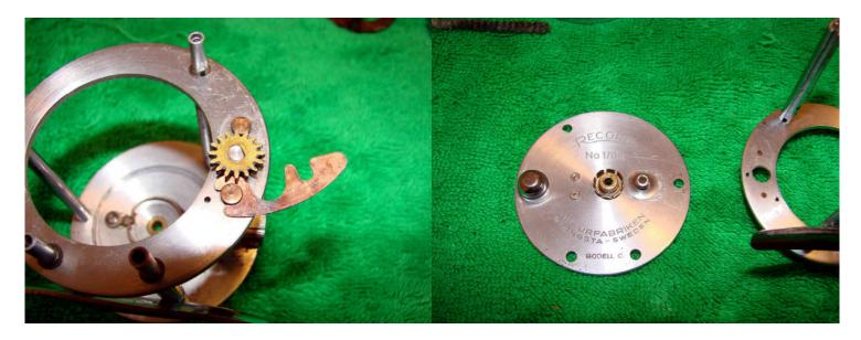
Slide off the locking washer-the worm gear can then be removed from the side of the frame. If you remove the four screws holding on the left side plate this lifts off. The worm cover can then be removed.
