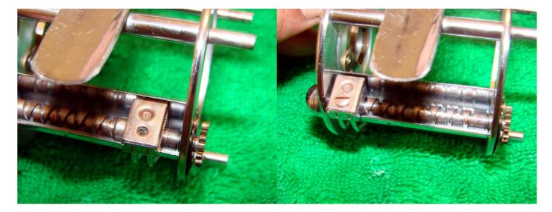
Replace the pawl cover and screw (greased threads naturally!).
