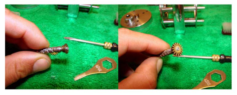
The gear cog on the end of the worm gear pulls off. Remove the bushing and place liquid grease where it contacts the worm gear. Replace the bushing and then press the cog back on to the worm gear so it is a snug fit.
