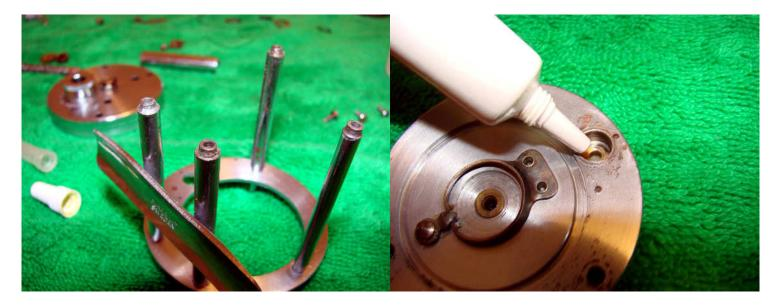
Before reattaching the side plate it is a good idea to place a thin smear of grease to posts where they contact the side plate. Add a drop of oil to the worm gear cap in the left side plate before reattaching the side plates. Don't forget to grease the screw threads. There are two holes in both side plates where the worm gear cover sits.
