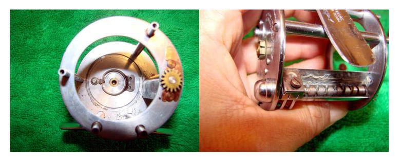
The locking washer for the worm gear-the design hasn't changed on present day Ambassadeurs. To remove the line carriage (level wind), first unscrew the screw holding on the plate at the base of the level wind.
