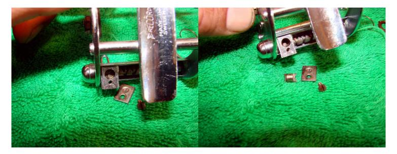
Remove the plate for access to the pawl, this can be removed with a pair of tweezers. Note it is 'double ended'-when one side wears out you simply flip it over-ingenious!
