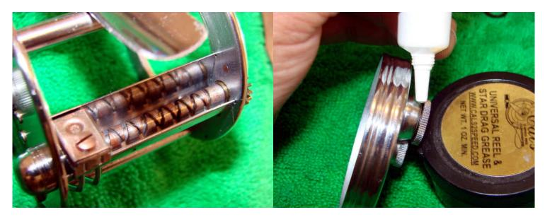
Place liquid grease on the entire worm gear-not just in the threads-the level wind is supported by the worm gear (unlike modern Ambassadeurs where it is supported by the worm gear cover). Add a drop of oil or liquid grease to the base of the crank ring (?) when it is fully screwed out. Screw it in and out a few times to ensure proper coverage.
