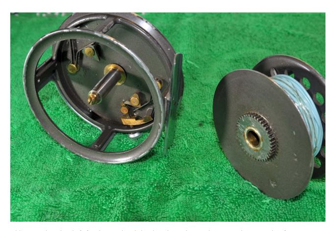
Add some oil to the shaft for the spool and the threads on the spool tension adjuster. Other friction points including the gear teeth get a very light coat of grease. Replace the spool in the frame and add a drop of oil to the handle.
