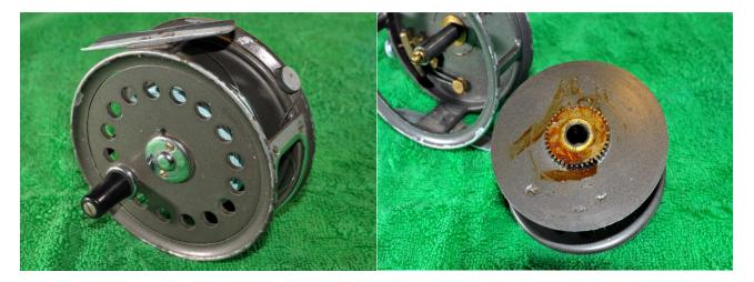
Remove the spool by pushing the chrome lever in the spool centre and then lifting the spool off. Apart from some old dried on grease everything looks fine.
