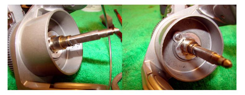
Note there is a rubber o-ring missing. Remove the rotor nut lock plate screw and the rotor nut lock plate.
