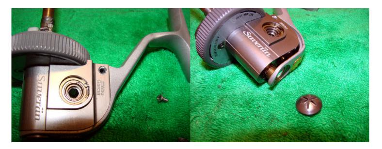
Undo the two screws holding the gearbox to the body (one either side) and then remove the screw securing the main shaft to the body.
