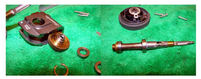
And then remove the bearings and main gear. The main shaft and pinion gear can then be removed.
