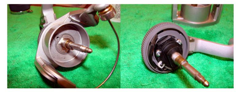
Undo the rotor nut and lift off the rotor.
