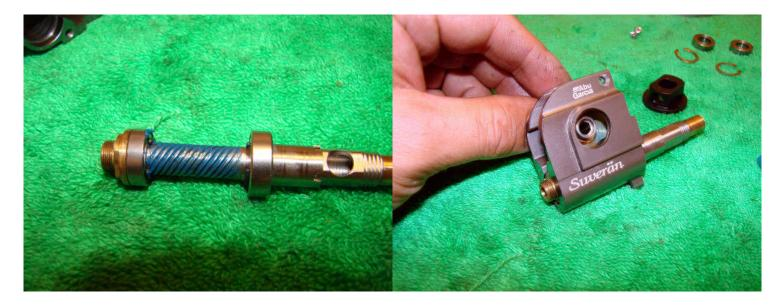
Clean and then lubricate all the bearings with a light grease (I use liquid grease). Grease the pinion gear and the main gear and then replace in the gearbox.
