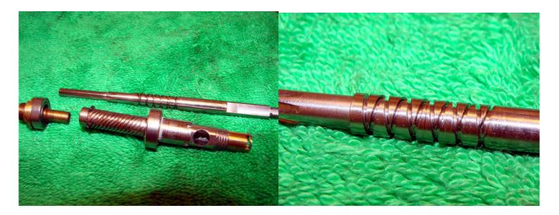
Remove the main shaft from the pinion gear-note the damage to the worm gear on the main shaft (teeth on far right). It looks as though the pawl and worm gear were jammed at some stage-the pawl is the only part holding the main shaft in the body and it is likely that a combination of a heavy drag and low stretch braid caused this problem.
