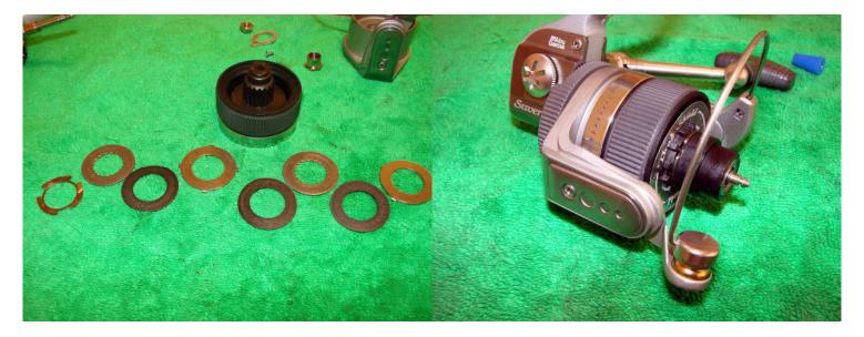
Separate out drag washers (left to right = bottom to top). Thoroughly clean the washers with a clean cloth soaked in lighter fluid. I don't have much faith in the drag shield and so I have greased the clean fiber washers with drag grease (Cal's drag grease). Replace the drag washers in the correct sequence and replace the upper spool bushing.
