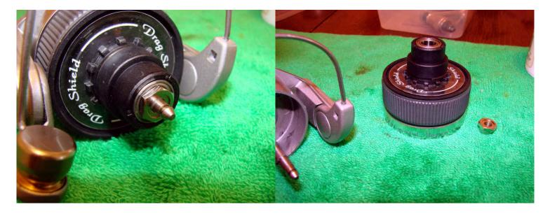
Remove the nut at the end of the main shaft and remove the entire drag system. Put this to one side to be worked on later.
