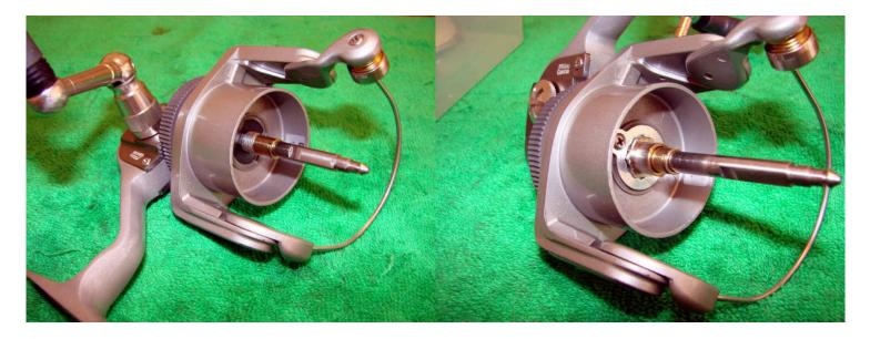
Replace the rotor (note that you have to line up the pawl assembly with a slot underneath the rotor). Replace the rotor nut, rotor nut lock plate, and rotor nut lock plate screw.
