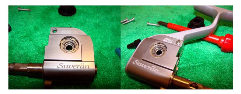
After cleaning and lubricating the bearings replace them in the gearbox and fix in place with the circlips. Replace the gearbox in the reel body and replace the two screws holding it in place.
