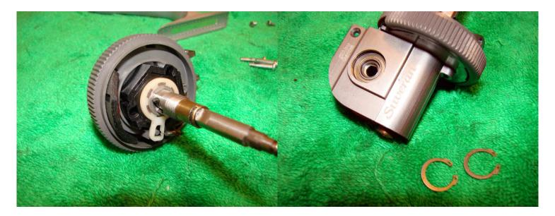
The reel body and the complete anti-reverse assembly can then be removed. Remove the bearing circlips.
