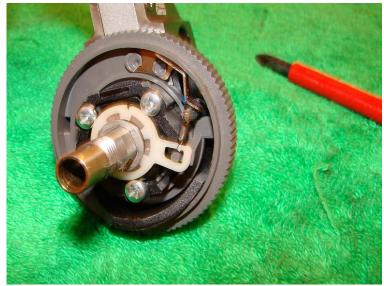
and replace the three screws to fix it in place.
