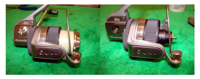
When this Suverän came to me it appeared to have a major problem-the spool did not move in and out when reeling the handle. As line lay is controlled by a worm gear and pawl I suspected that these were damaged. Overall the rest of the reel was in very nice working condition though.
