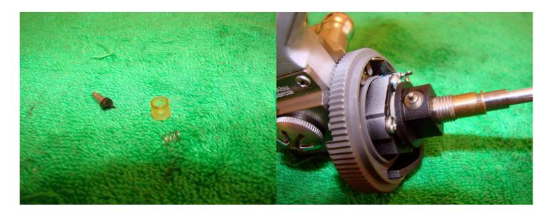
These are the replacement parts-pawl, pawl sleeve and pawl spring. These fit in the pawl holder that sits on the pinion gear. Before replacing the pawl assembly, lightly grease the main shaft (liquid grease or heavy oil) and slide it into the pinion gear. Then slide on the pawl holder and finally insert the pawl, pawl spring and pawl sleeve into the holder.
