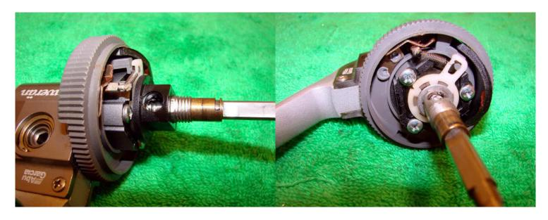
This seems to be the problem with the lack of line lay-the pawl is missing completely. Remove the pawl holder and then remove the three screws holding the anti reverse selector to the body.
