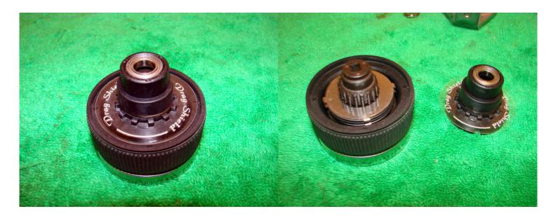
Remove the upper spool bushing (this contains the bearing and drag shield). Thoroughly clean the bearing and lubricate with light grease.
