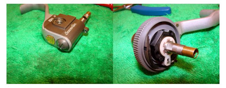
Grease the threads on the shaft nut and then replace. Replace the anti reverse assembly on the gearbox
